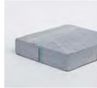
**Material** Sand, Zement, Kalk, Gips, Wasser
